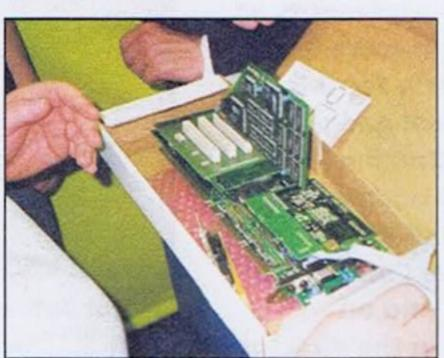
The board will only work in a Zorro IIIequipped Amiga due to the fact that the 8Mb of RAM on the board will take up the entire Zorro II memory map, without taking into account the additional 4Mb of memory that the PicassoIV board itself
