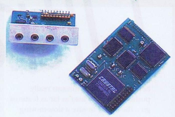
On the hardware front the Prelude 1200 has CDROM audio, MIC, Line and Auxiliary inputs. The supplied graphical mixer software allows non-retargetable Amiga audio to be properly mixed with the output from the Prelude card for a single connection to your HiFi or speakers.
